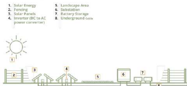
Components of a typical solar farm
